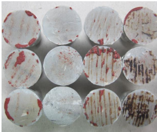
Aluminum Dollies after Pull Off Test Demonstrating Cohesive Failure
