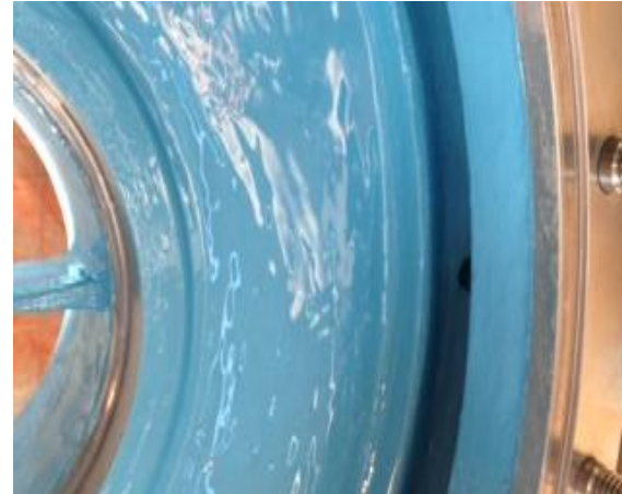
Repair: Seawater pump Rebuild & protective coating
