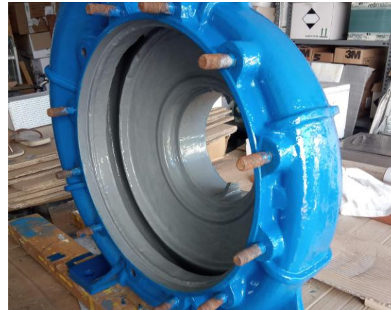
Repair: Seawater pump Rebuild & protective coating
