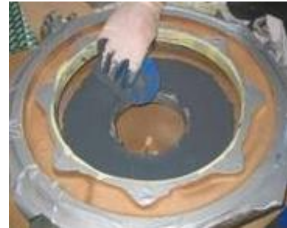
Repair: Seawater pump Rebuild & protective coating
