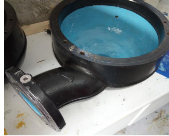
Repair: Saltwater sea pump Rebuild & protective coating
