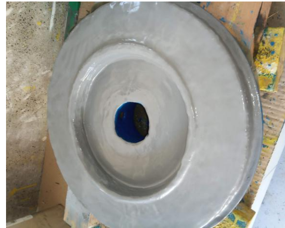
Repair: Seawater pump components Rebuild & protective coating
