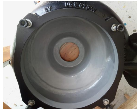
Repair: Seawater pump Rebuild & protective coating
