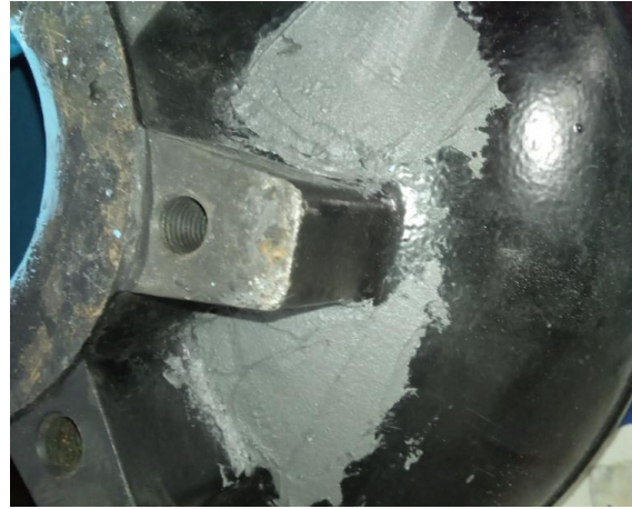
Repair: Saltwater sea pump Rebuild & protective coating
