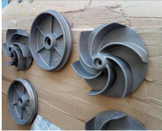
Repair: Seawater pump components Rebuild & protective coating
