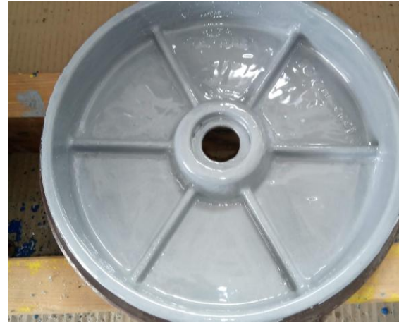
Repair: Seawater pump components Rebuild & protective coating
