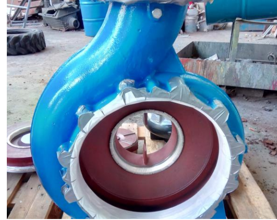
Repair: Seawater pump Rebuild & protective coating
