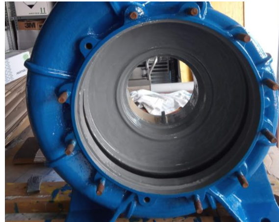
Repair: Seawater pump Rebuild & protective coating
